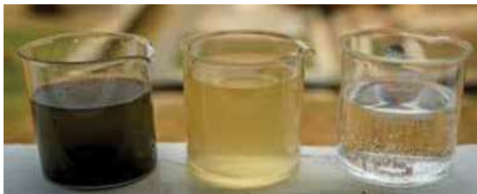
Figure 4: Raw Sewage, After Bio-Filter and After Membrane quality water
